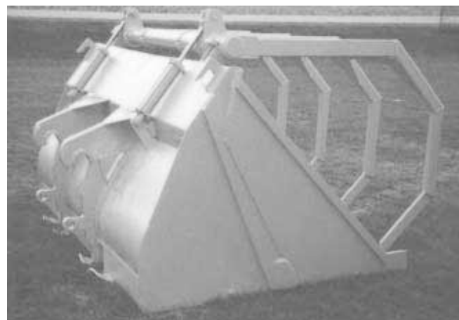
Therkilsen doubled the width of bucket to 68 in. and added a grapple fork.
