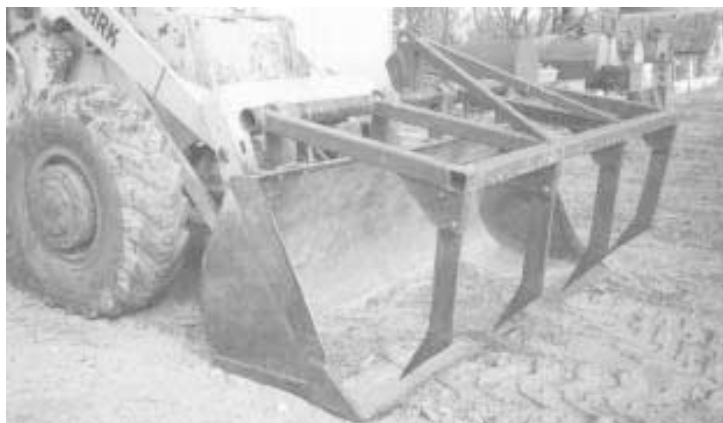
Rectangular frame supports four forks made of 4-in. wide, 3/4-in. thick flat iron.
