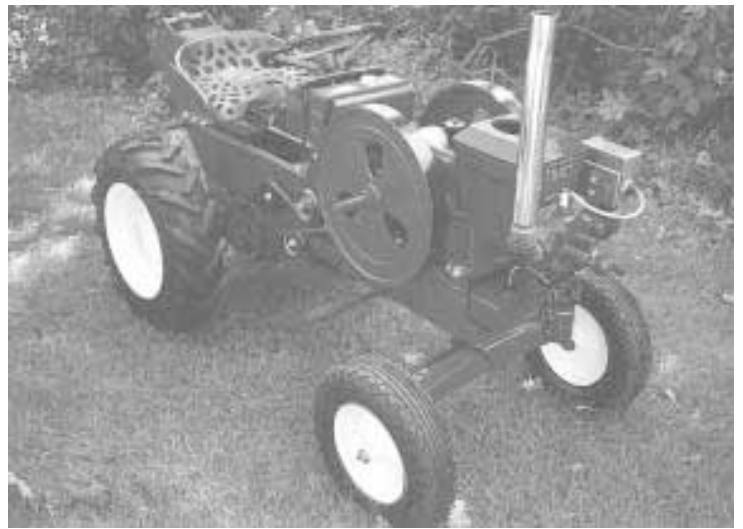
Wheelhorse tractor is powered by a Stover-Built "Economy" engine that's equipped with an open-topped radiator on front to keep the engine cool.
