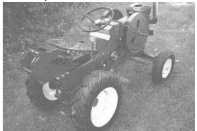
Pulley mounts on one of the engine's flywheels to belt-drive the original transmission.
