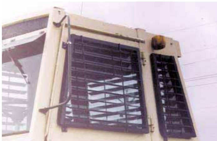
Homemade sun shades are made from lengths of 2-in. wide strap iron welded at an angle to metal rods. They cover all five window's on Stout's tractor cab.
