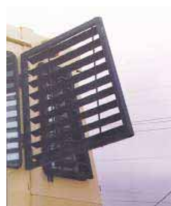
Stout welded a pair of hinges to each frame so they pivot out as needed to clean windows.
