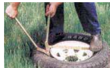
Australian-designed bead breaker is a three-levered scissors-type tool that can be used on any rim - alloy or steel - without damaging the rim or sidewall.
