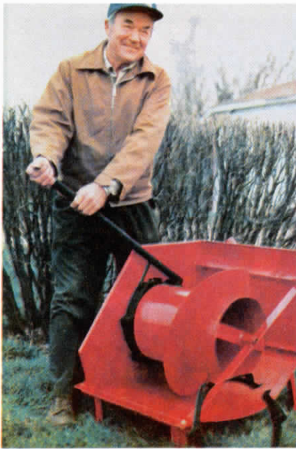
"Unplugging" ring bolts onto auger.
