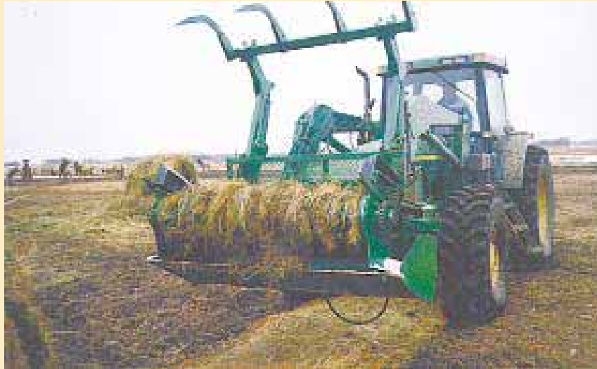
"It works great for stripping twine off big round bales," says Allen Schwitzer about his "Twine Stripper" which fits inside a front-end loader bucket. Powered drum is driven by two orbit motors. When pressed against the side of a bale, the drum strips twine off and wraps it up.
