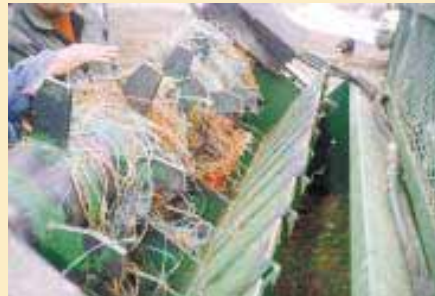
Cutting blades drop down against drum as needed to effortlessly remove the rolled-up twine.
