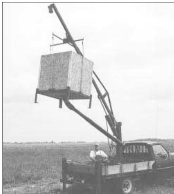
Home-built boom can lift 1 ton of seed up to 28 ft. high.
