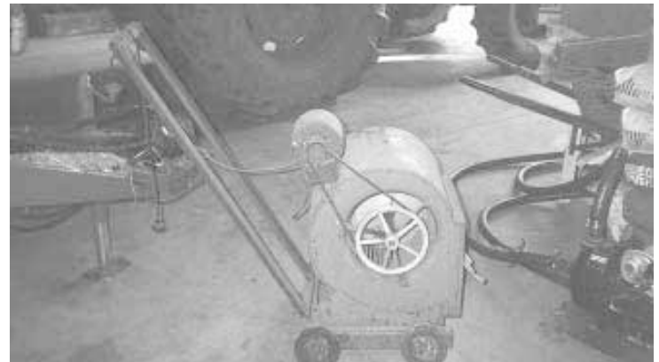
Fan mounts on angle iron frame equipped with lawn mower wheels and push handle.
