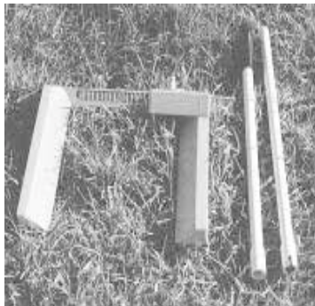
Clark made chock to keep his airplane stationary inside hangar.
