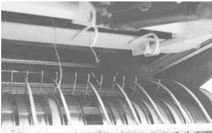
Hydraulically-operated 4-in. hooks push hay and weedy material through pickup (see arrows).
