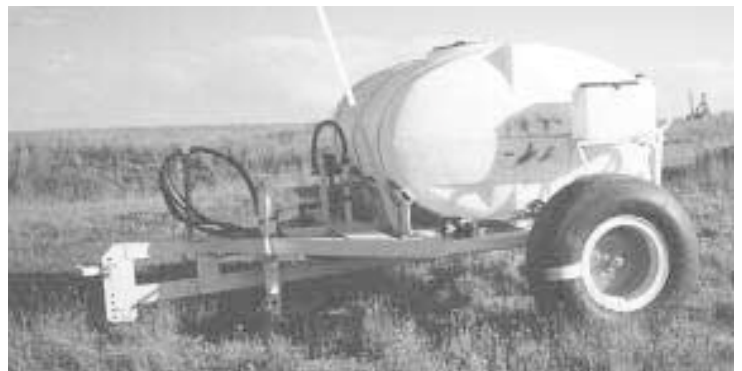
Cart's homemade frame and axle, which is equipped with flotation tires designed for World War II "bomber" airplanes, carries a 1,500-gal. poly tank.
