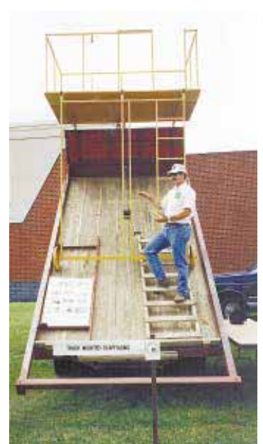
When mounted on a 16-ft. long truck bed, the scaffold reaches up to 21 ft. high.
