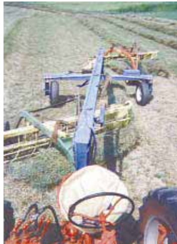
“Swing” mower’s bridge hitch and the hydraulic cylinder on it were left intact.
