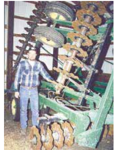
Wavy coulters mounted on his 24 1/2-ft. disk dry out wet soils, allowing Buzzard to plant no-till beans earlier than he ever could before.
