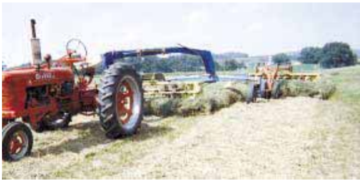
Hitch allows Spoerl to pull a 9-ft. Deere 670 and New Holland 258 rake together.
