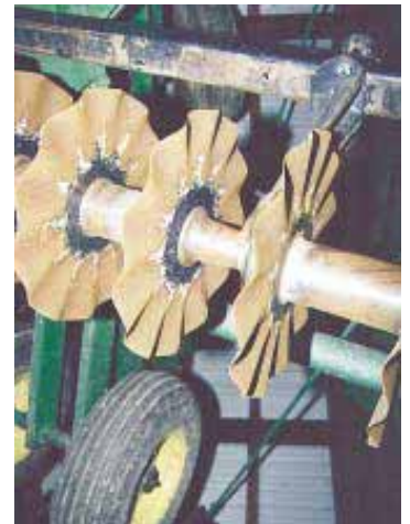
Spaced 9 in. apart and offset on two gangs, the 20-in. dia., 1 7/8-in. coulters were modified at the factory to mount on the disk’s square shaft.
