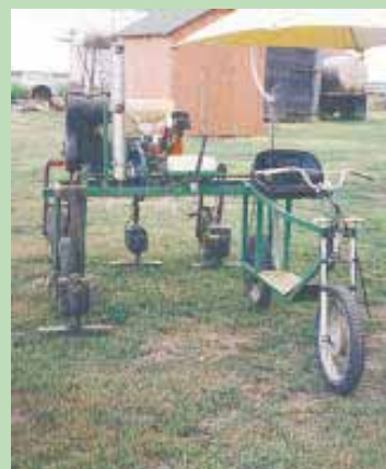
Blades are set to run 1 1/2 in. above the ground.
