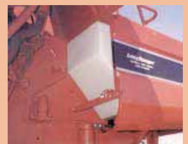
Add-on 36-gal. poly gas tank slides in next to the original 100-gal. fuel tank, under the outer shell of the combine.
