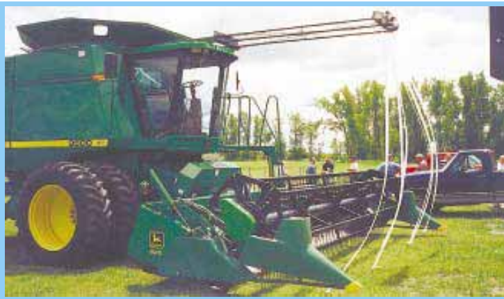
Extension bracket puts lights out in front of header for better visibility. Paper streamers hanging from light in photo show where light hits.
