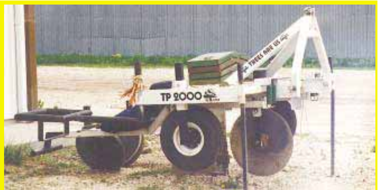
Tree planter is equipped with a pair of 16-in. dia. steel wheels that weigh 45 lbs. apiece.
