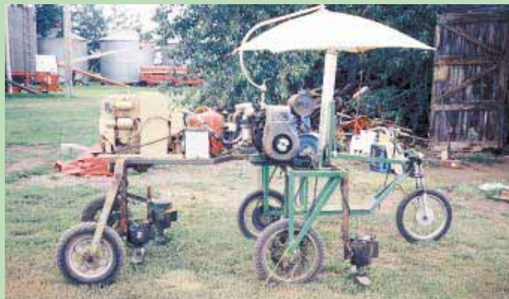
Three 3/4 hp electric motors fitted with 19-in. long blades are powered by a generator.
