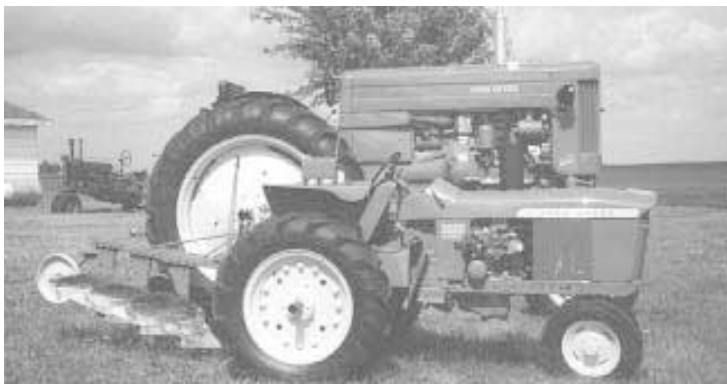
Controlled by a model airplane radio remote, the mini 3020 is powered by a Yanmar diesel.
