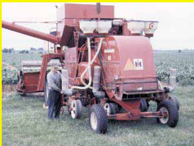
Seed was blown to planter units by individual air-powered units - one per row.
