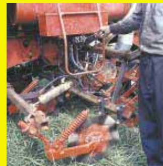
White planter units were mounted on a toolbar that ran under the back of the International combine.
