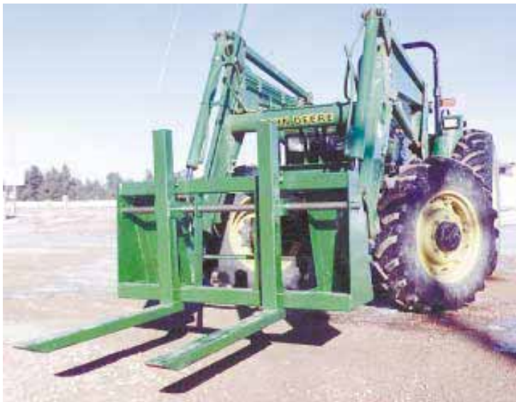
Brecht copied Deere’s basic pallet fork design but beefed it up.
