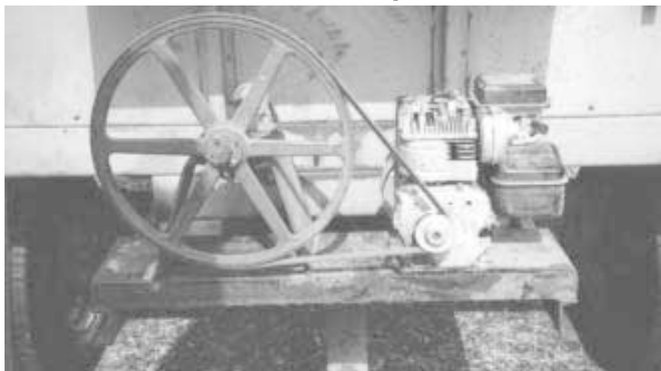
Frick mounted a 5 hp gas engine on front of wagon. To unload all he has to do is pull-start engine. No more hitching and unhitching wagons to hook up the pto.
