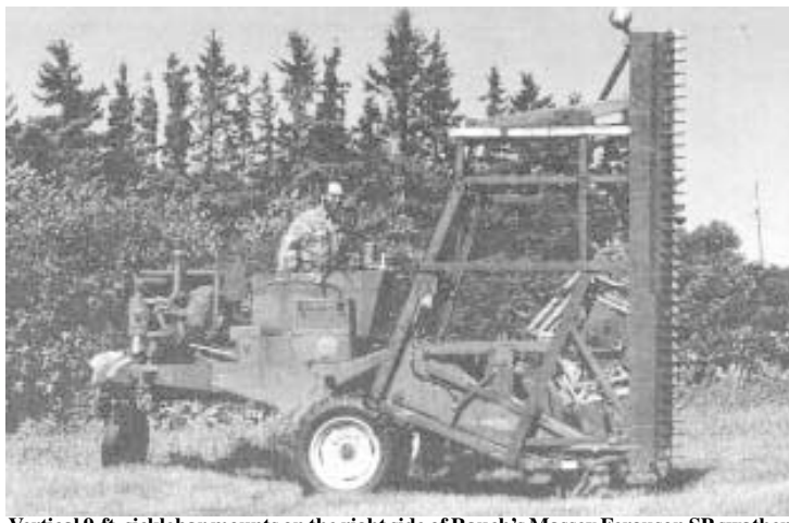
Vertical 9-ft. sicklebar mounts on the right side of Rauch's Massey Ferguson SP swather.
