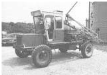
Ambulance sprayer can cruise at highway speeds of up to 65 mph. It's fitted with the cab off a 915 IHC combine.
