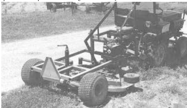
Mower attaches to 3-pt. tractor hitch and is fitted with flotation tires on back that let McKee mow in even the muddiest conditions around his fruit and vegetable farm.
