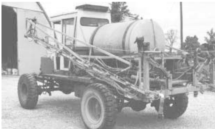
Sprayer's 60-ft. boom and 500-gal. spray tank came off an Ag-Chem sprayer.
