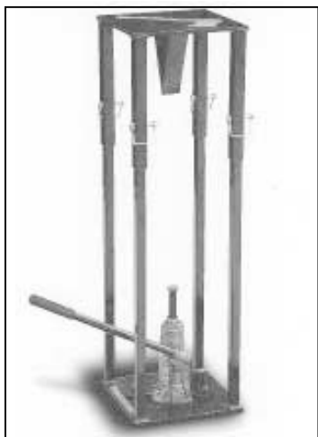
"Hand-pump" splitter is powered by a standard 6-ton bottle jack that pushes wood up into wedge.
