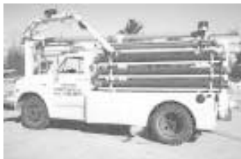
Wood converted a 1967 Chevy 4-WD truck into a pump truck equipped with a swing boom on front that fills a tanker truck.
