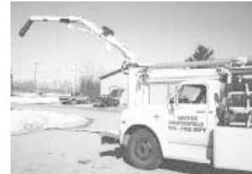
Boom rotates back and forth and moves up and down, controlled by hydraulics off a pto-driven hydraulic pump.
