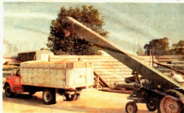
Hydraulic hoist at front of tractor raises and lowers the high-capacity conveyor.
