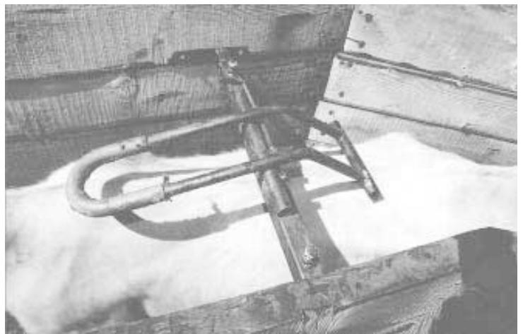
Tailgate is mounted at height of animals' backs so when they approach, they lower their heads and push up on U-shaped, rubber-covered bar.
