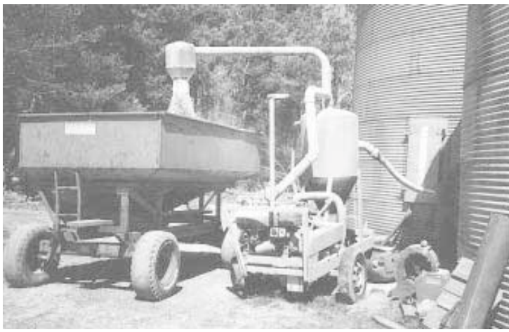
Larson's 3-wheeled, home-built grain vac sits on a channel iron frame that mounts above a car axle. Power is supplied by a 3-cyl. diesel engine.
