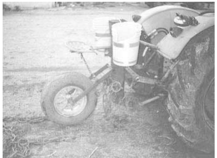
Planter rides on a single wheel with a tractor seat mounted above it for the operator. The operator drops seed potatoes by hand into a hollow 4-ft. long shank.
