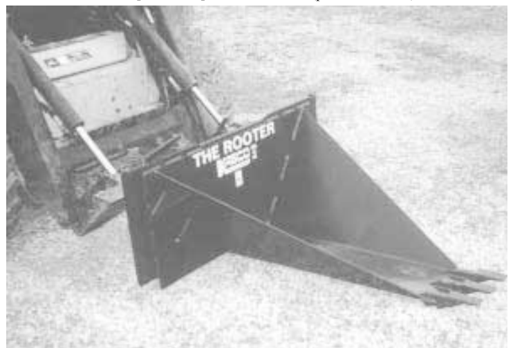
Rooter uses three backhoe bucket-type teeth on front to dig out trees or shrubs. It flares out to 36 in. wide at the top and is 3 ft. long from front to back.
