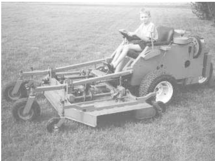
Mower deck has four blades belt-driven by two jack shafts, one on each side. Grass is discharged from both sides of mower.
