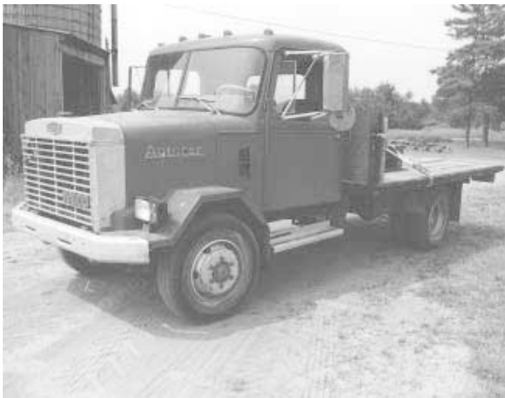
Larson restored his 1984 Iveco cab-over truck by replacing the truck's original cab, which had rusted out, with one off a used Autocar truck.
