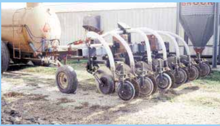
The Krofts pull their home-built manure applicator behind their honey wagon. Applicator mounts on the frame of an old DMI pull-type chisel plow.
