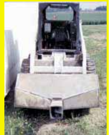
An 18-in. piece of rubber inner tube (tucked inside the opening in photo) adds length and helps direct seed.
