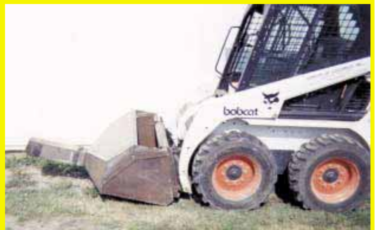
Modified skid steer loader bucket has a 2-ft. long chute with a 6-in. sq. opening. A sliding door over the opening controls the flow of seed.
