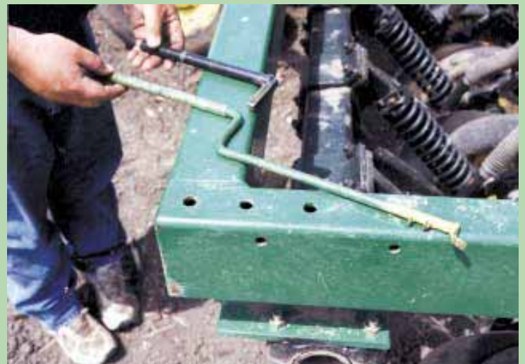
Home-built tool is much longer than the Deere tool, allowing Heaton to adjust both front and back units on his 750 grain drill from a standing position.
