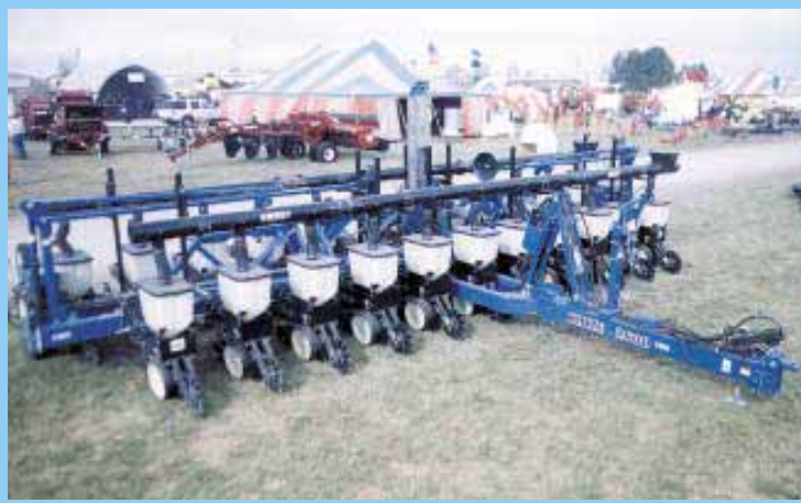
Filling Kinze's Twin-Line planter with seed goes a lot faster with Kasco's hydraulic-powered, double cross auger. It mounts permanently on the planter.
