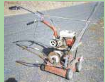
Rototiller, with the tines removed, mounts on the deck of a push mower frame. The rope on the walking pole wraps around a steel drum and bearing that Storla mounted on the rototiller shaft.
