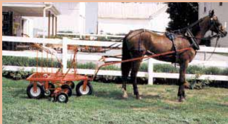
Horse-pulled rig uses gangs of ground-driven reel mowers attached to a single support arm and operating lever. Mower can also be pulled by an ATV or garden tractor.
