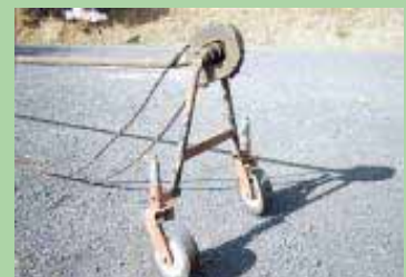
Two-wheeled "dolly" with a pulley mounts at upper end of walking pole. Rope runs over pulley and down to mower deck.
