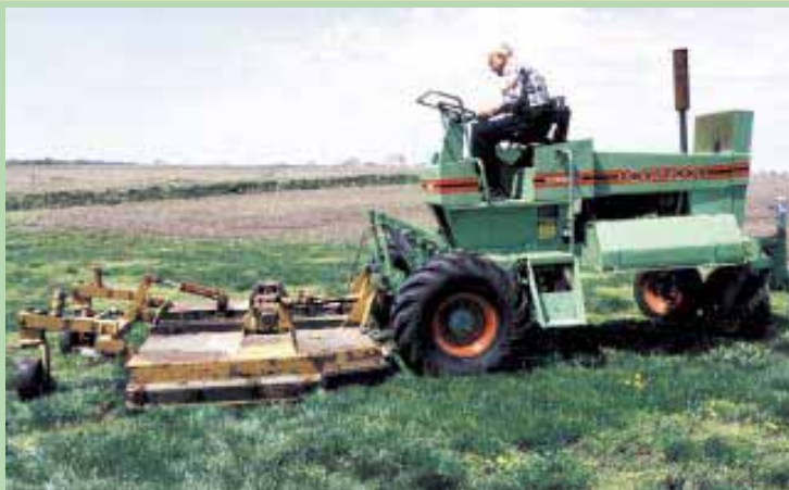
The mower deck is 2-point mounted to the swather.
