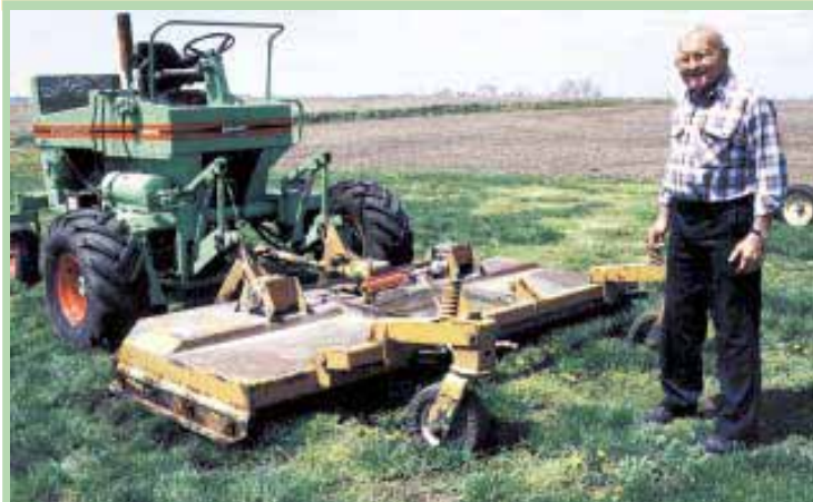
Butch Uhnken turned an Owatonna hydrostatic-drive swather into this big self-propelled mower with a 10-ft. Woods cutting deck.
