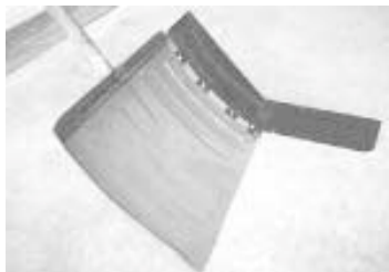
Schiltz also fitted a side shield to a standard snow shovel. A 4-in. high metal strip is bolted to side of shovel; another metal strip bolts across the top.
