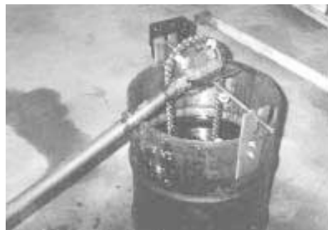
Bennett started with a 30-gal. drum which is filled with oil. A loop of roller chain hangs from a sprocket, with the lower end dangling loosely in the oil.
