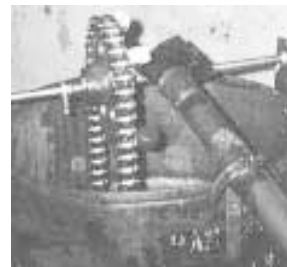
Caps from 20-oz. pop bottles are attached to chain, which is turned by a motor. The caps act as little buckets for dipping up oil.
