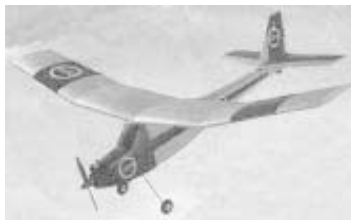
Hand-launched reconnaissance plane takes a single mid-air photograph and lands by itself.
