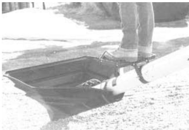
Auger step clamps onto auger, just above hopper tub.
