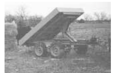
Two lengths of heavy channel iron run lengthwise across the top of the axles. A 12-volt hydraulic pump mounts at the front of the frame.
