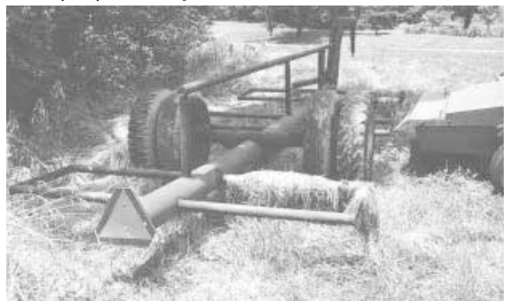
A length of 8-in. dia. pipe runs down the middle of the trailer, with three rectangular bale carriers welded onto each side.
