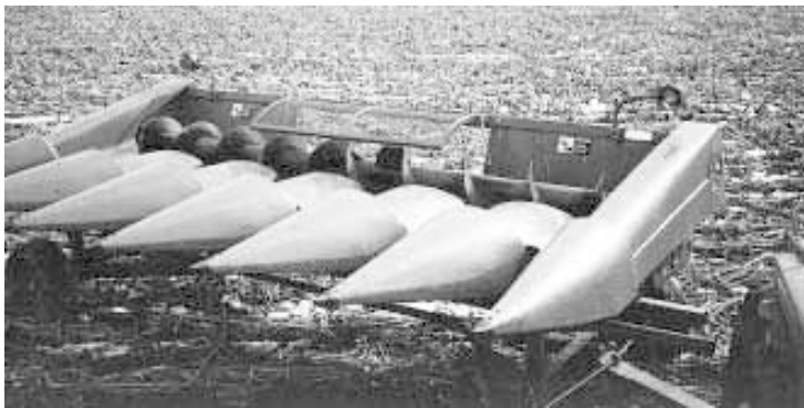
The cob saver is designed for smaller, newer Deere headers with high-speed augers.
