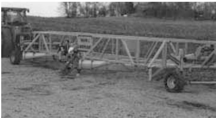
Dodd has greatly improved drainage on 80 acres with his land plane, traveling diagonally across the field on the first pass, then going the opposite direction on the second.
