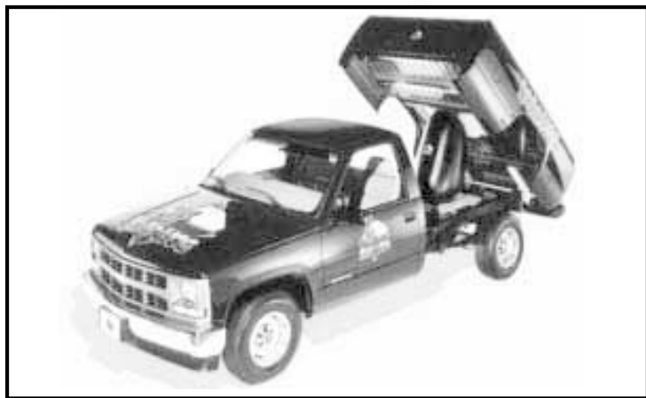
Kit allows a standard-size pickup to dump up to 4,500 lbs. to an angle of 50 degrees.
