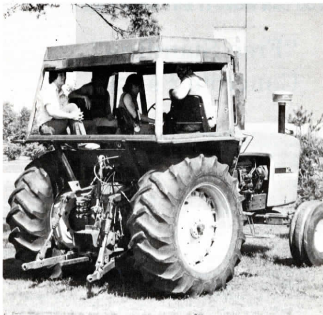
Multi-passenger cab developed by Iowa State University Agricultural Engineers comfortably seats driver and 2 or 3 passengers.
