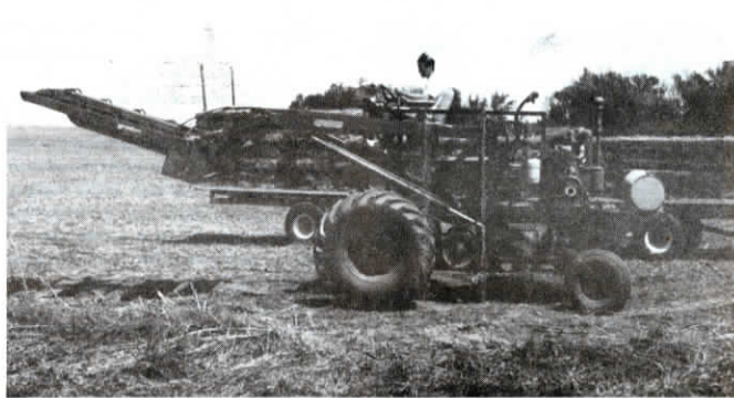
Keeler mounted used Farmhand F11 loader and bale fork on old Gleaner combine.
