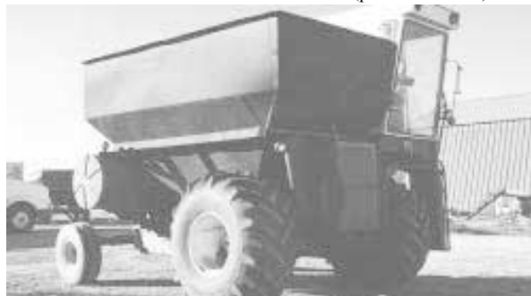
A 400 to 450-bu. grain box was fashioned out of sheet steel and mounted on the right side of the cab.
