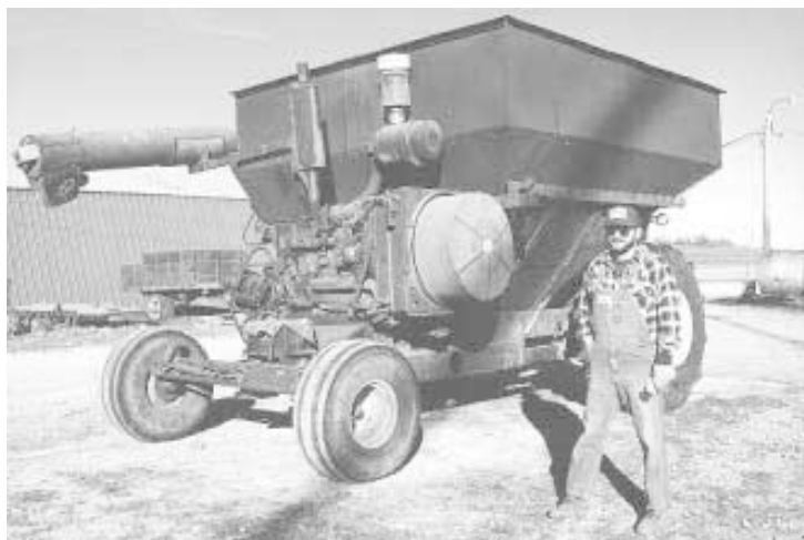
Engine was lowered 6 ft. and remounted on original combine rails to ensure the unloading auger would clear the engine.
