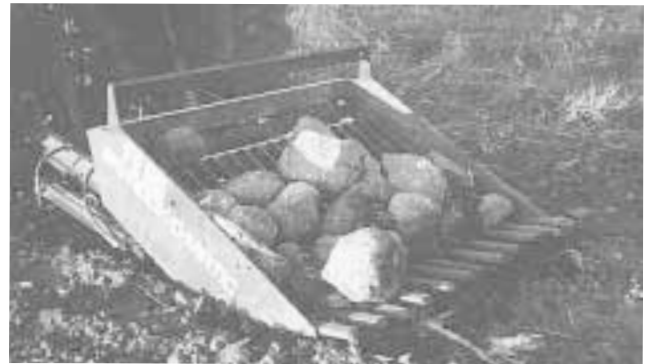
Dan Wagner and his father converted this commercial loader-mounted rock bucket to a 3-pt. model they say is much easier to see from the tractor cab.
