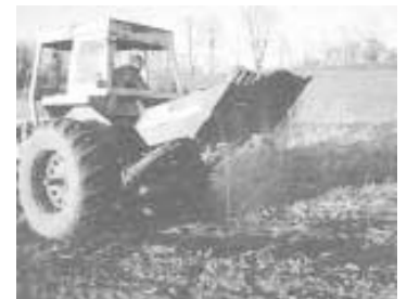
Bucket lifts high enough to dump into a pile several feet high.
