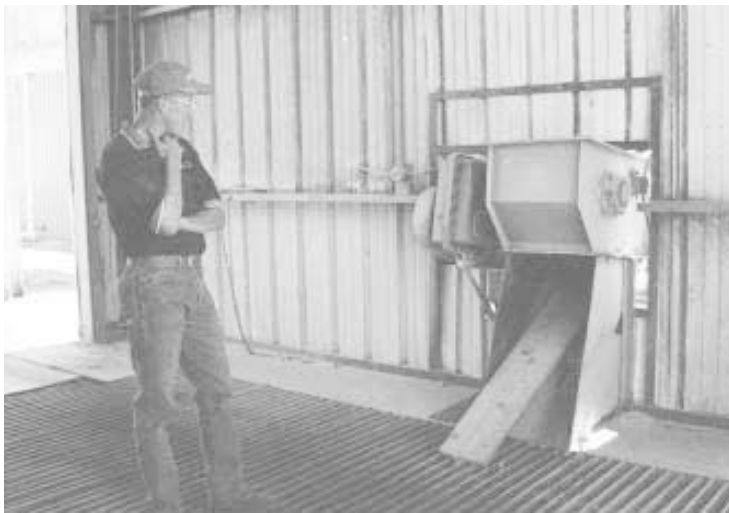
Lyons positions large pieces of wood at a 45 degree angle under unloading chutes on rail cars. It takes about 10 rail cars or 30,000 bu. of wheat to sand a 4-ft. long board.
