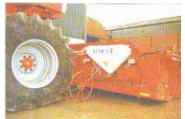
Ground-driven "Autocast" system mounts behind combine header and consists of a hopper, electric fan, and outlet nozzles.
