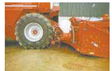
A ground-driven wheel meters the seed.
