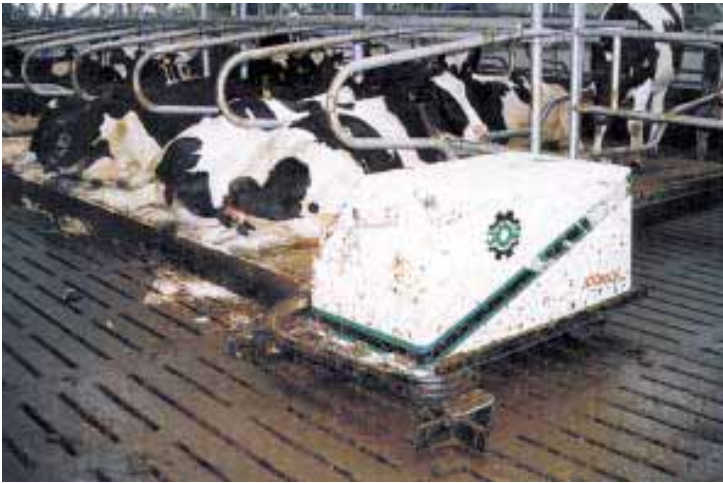
Moving at a slow crawl, battery-powered robot uses front-mounted rubber squeegees to scrape away manure.
