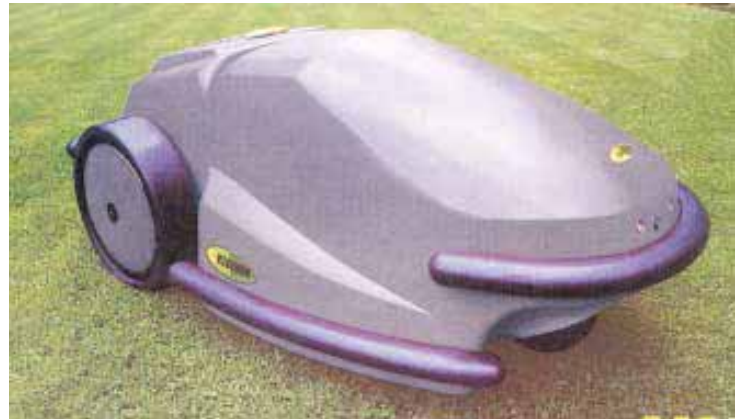
Electric-powered "Robomow" senses the height of the grass and cuts only when necessary. It senses obstacles and works its way around them.
