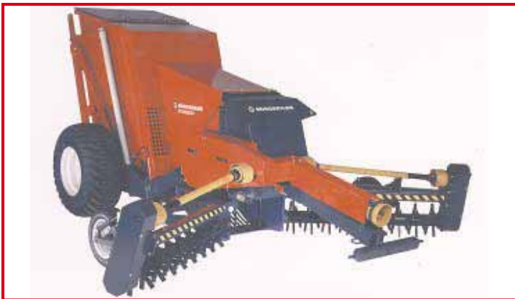
Pto-driven rock rake is equipped with raking fingers that work down to about 6 in. deep, pulling rocks to the surface and then windrowing them.
