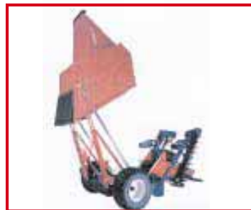
Entire rear rock box lifts up high via 6-ft. cylinders to dump rocks.
