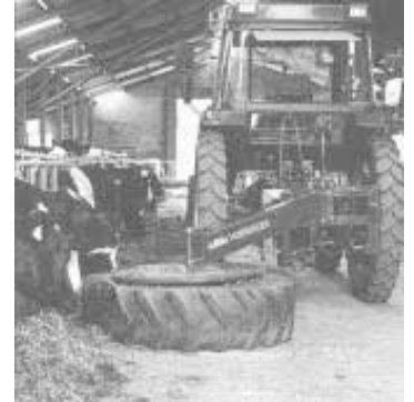
Tire bolts to a steel plate that rotates at the end of a 3-pt. mounted steel arm. Works great for keeping feed within reach of cattle.
