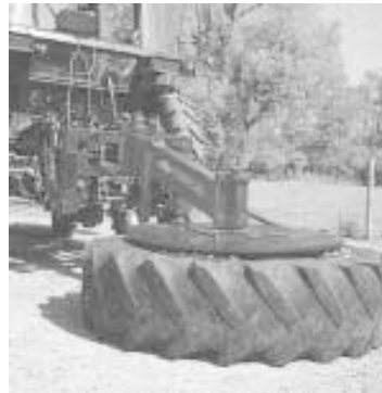
Tire bolts to a steel plate that rotates at the end of a 3-pt. mounted steel arm. Works great for keeping feed within reach of cattle.
