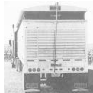
Extension consists of a bellows-type frame that bolts to trailer top.
