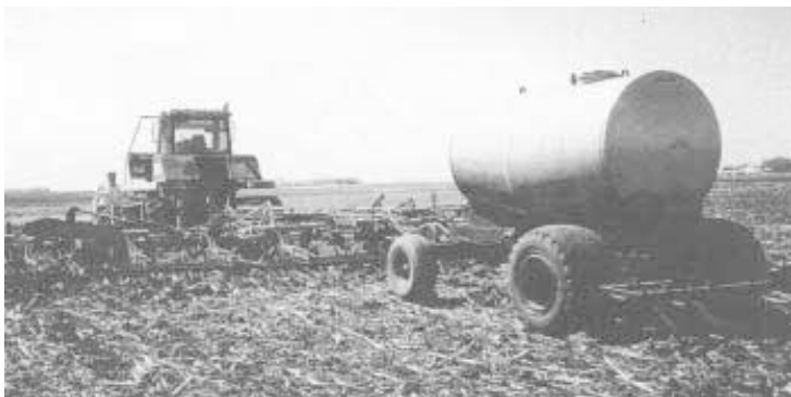
Oftedal's rig lets him safely carry 1,250 gal. of herbicide without saddle tanks or other add-on equipment.
