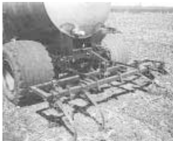
Applicator consists of a field cultivator, spray boom and trailing tank.
