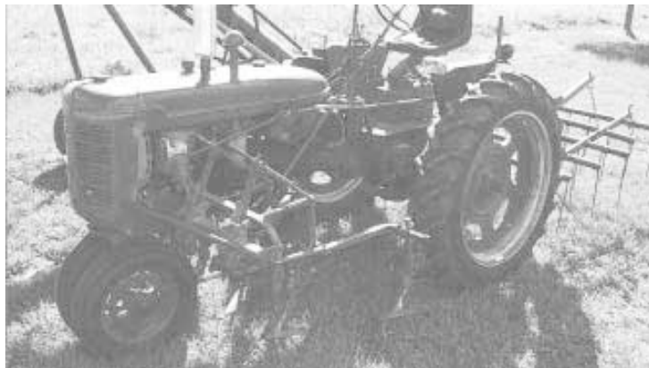
Goodall narrowed up a 2-row, 40-in. cultivator to fit his 30-in. rows.
