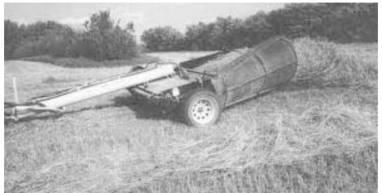
ReCon 200 hay conditioner is equipped with a pair of 12-in. dia. steel rollers on front and a pair of curved, 8-ft. long poly deflectors behind them.
