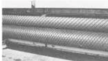
Heavy duty rubber-coated steel rollers are held tightly together by an air bag pressure system.
