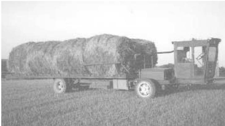
Ballard's bale hauler is equipped with a loading arm that picks up bales on-the-go. It's built out of an IH truck frame and combine cab and powered by a car engine.
