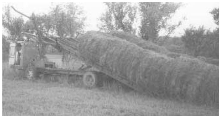
To unload bales, the operator hydraulically tilts the bed until the back end touches the ground and then pushes bales off as truck moves ahead.
