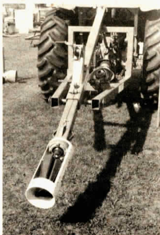
Cutaway shows how folded-up prop fits into 8-in. pipe.
