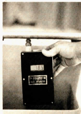
Operator holds digital tester over nozzle to test flow.
