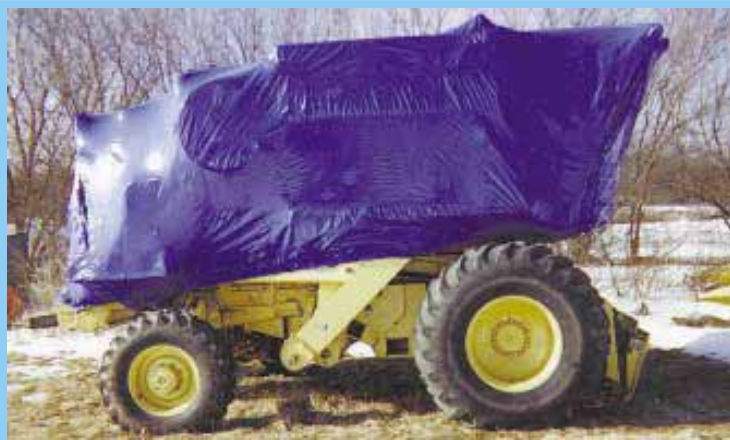
Heavy duty shrink-wrap plastic works great to protect combines, tractors and other equipment, says Bill Knoff.
