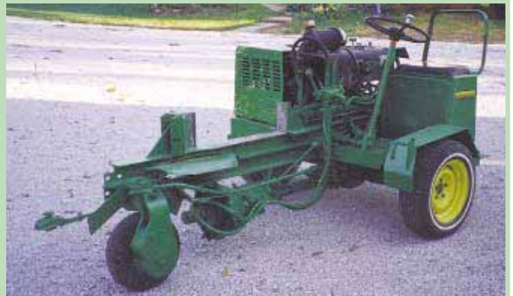
Boldebuck mounted an electric-start, 2-cyl. Wisconsin engine off an industrial sweeper on right side of rig, and the seat, gas tank, and steering box on left side.
