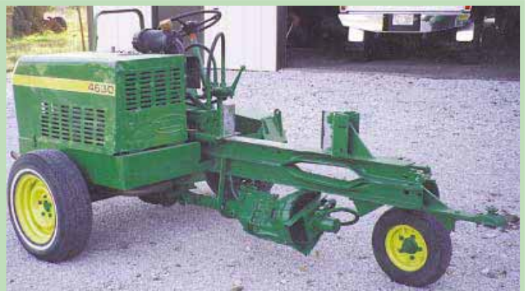
Boldebuck mounted his pull-type log splitter on a Ford car axle and fitted it with a single wheel up front that's used for steering.
