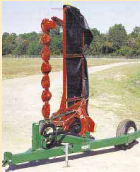
Two-wheeled "Hay Caddy" attaches permanently to rotary disc mowers, converting them to pull-type.
