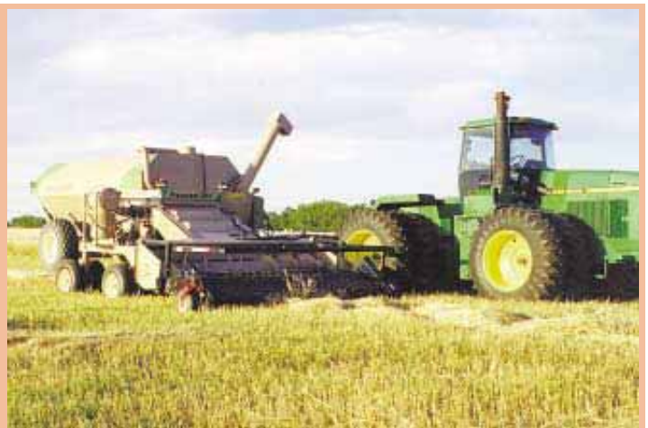
McLeod's harvest system includes a swather header mounted on the side of a tractor. Grain and crop residue, minus the straw, are blown into 1,200-bu. hopper.
