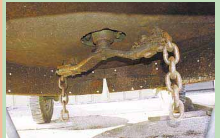
Each piece of chain is made up of six 3/4-in. links.
