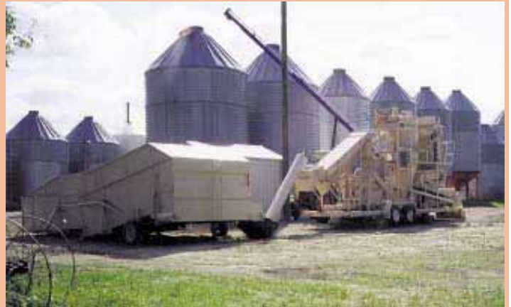
On-farm mill separates grain from crop material gathered in the field. Mill is powered by a 30 hp electric motor and handles up to 800 bu. hour.
