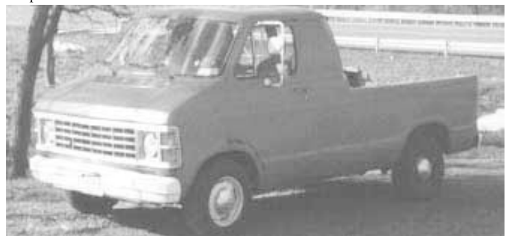
Wilbert’s pickup was converted from a 1983 Dodge Ram van. He cut off the back of the van and left 2-ft. high sides for the bed. He reinforced the bed sides and filled in the back of the cab with left over material.
