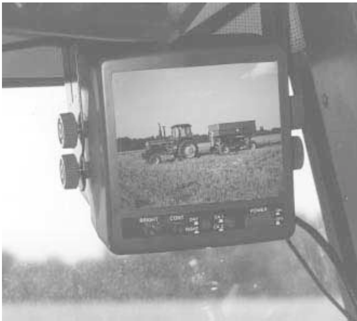
Photo shows monitor mounted inside a Deere 9500 combine.
