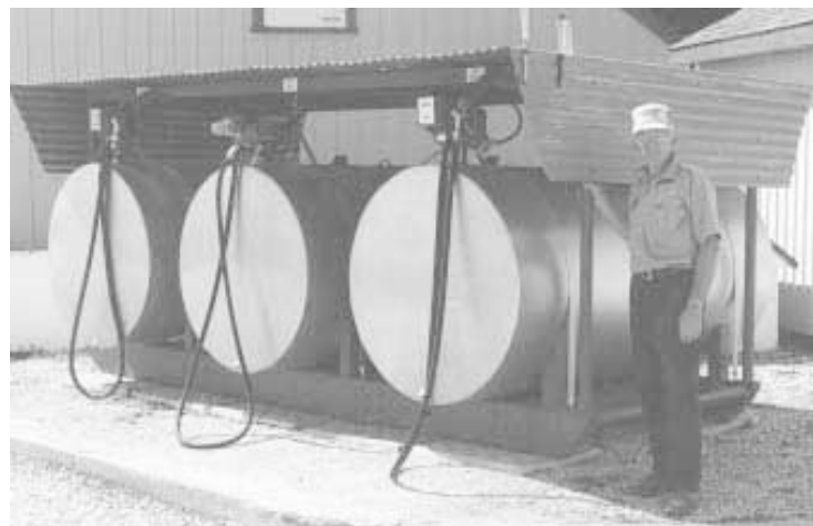
Semi truck frame was used to build the 15-ft. long by 5-ft. wide skid which holds three 500-gal. fuel tanks.
