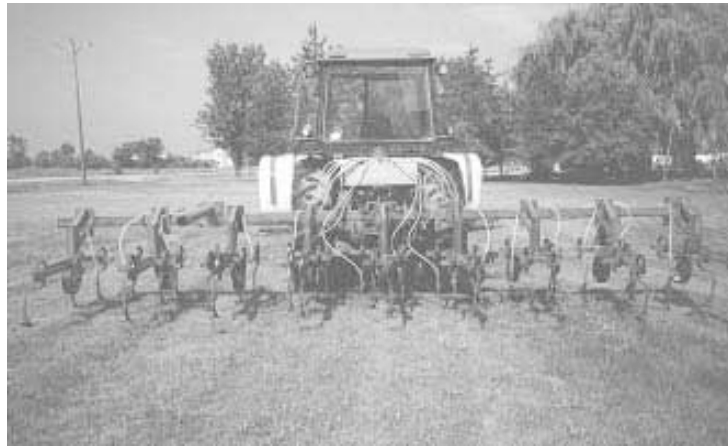
By mounting a liquid nitrogen applicator on an 8-row cultivator, Walton can do two jobs at once and save a pass through the field.
