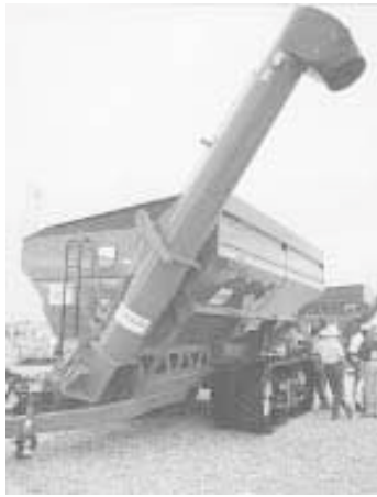
Dual-auger cart is equipped with a 20-in. dia. fold-out unloading auger on front and a horizontal auger at bottom.
