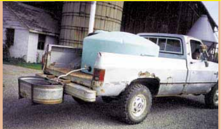
Horst mounted a 425-gal. poly spray tank on back of an old pickup. A 50-gal. stock tank mounts on pickup bumper.
