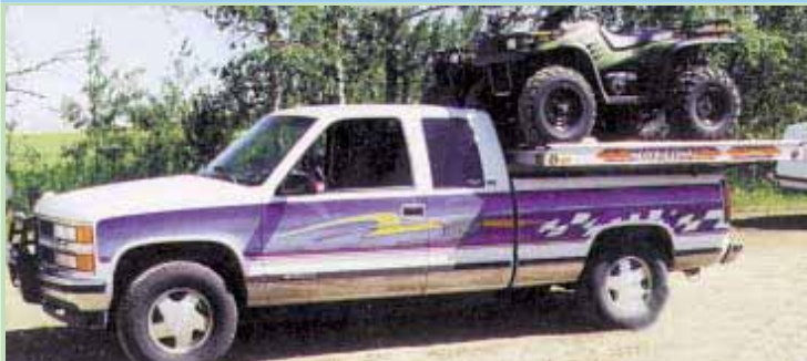
Tilting flatbed mounts on a subframe that slips inside pickup box and bolts to floor.
