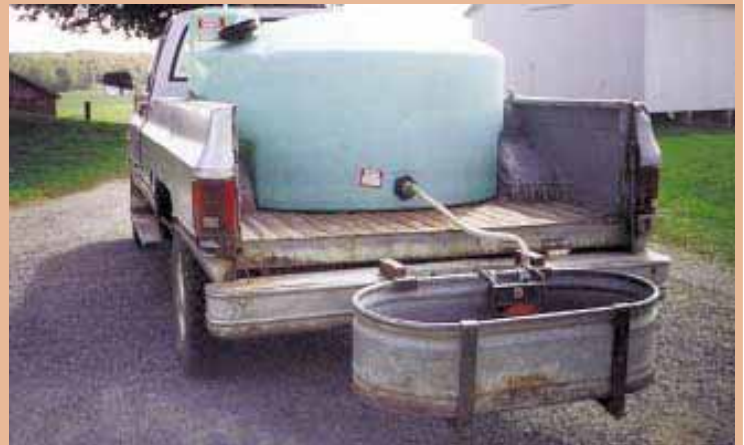
He put a float in the tank and built a guard around it. There's enough water to supply 35 cows for 24 hours.
