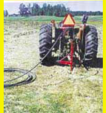
A 3/4-in. water line feeds into a pipe that mounts directly behind subsoiler shank.
