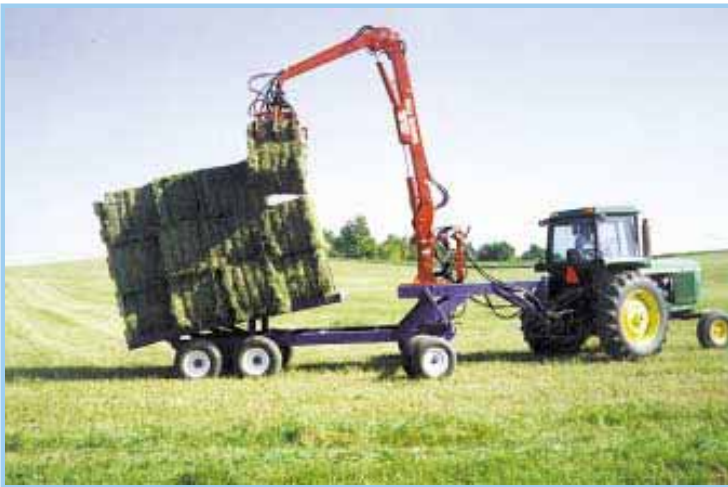
Loading boom pivots 240 degrees to load bales out to either side of trailer. It'll handle mid-size square bales, large square bales, round bales, and plastic-wrapped bales.
