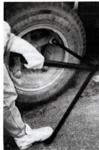
"Step-on" bracket and "cheater" wrench bar combine to provide extra leverage for loosening tight nuts.
