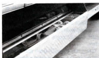
Top slips off to the side to reveal a 4 by 8-in. storage compartment that's as long as the running boards.
