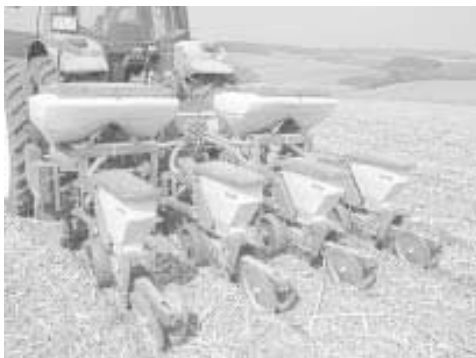
The Kverneland Accord Optima 3-pt. planter uses a high performance fan to provide the vacuum supply for up to 18 rows. The fan can be pto or hydraulic driven.
