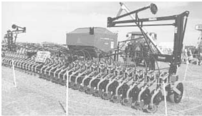
Hiniker's 4800 "row crop" air seeder cart has a 40-ft. toolbar and 130-bu. tank.
