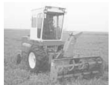
Pto-driven snowblower mounts on a 3-pt. hitch that bolts onto front axle. Both the front and rear axles were narrowed to put axles on 60-in. centers.
