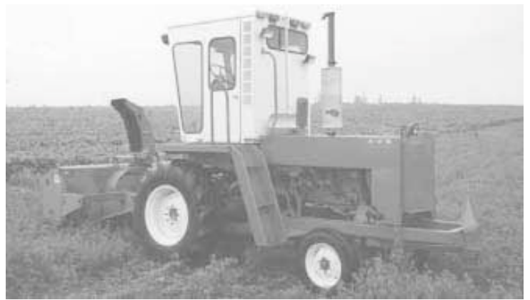
Basener mounted a 7-ft. 2-in. IH snowblower in place of the header on a stripped-down IH 615 combine.
