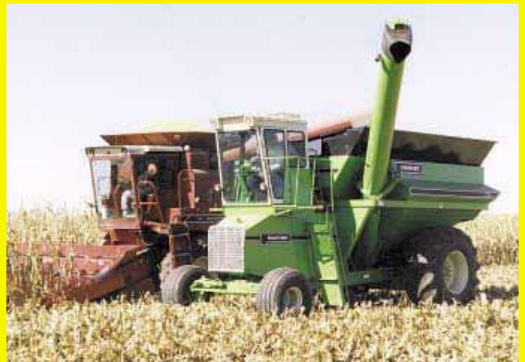
VanderLinden powered a Parker 710 grain cart with a 407 cu. in. diesel engine and hydrostatic drive out of a mid 1970's IH 915 combine. He also equipped the self-propelled cart with a combine cab.
