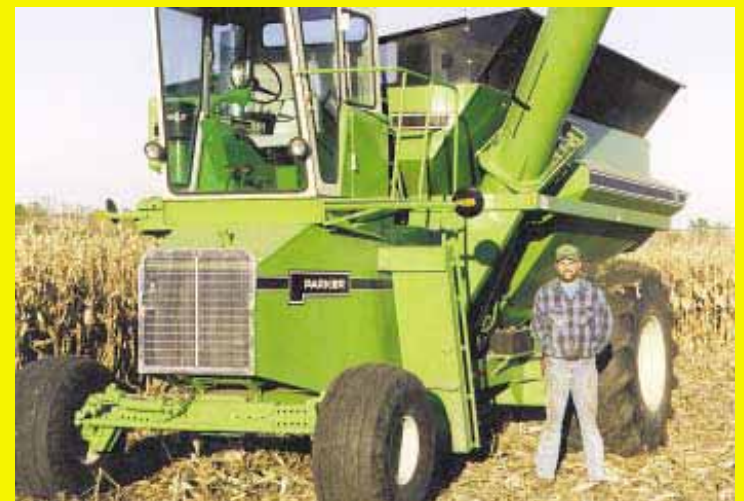
The rear 30.5 by 32-in. tires are taller than what they were on the 915 combine, which gives VanderLinden a faster ground speed and better flotation in the field.
