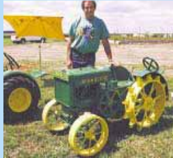
Prom's half-scale, steel-wheeled Deere Spoker D is powered by a 6 hp Kohler gas engine connected to a Wheelhorse transmission.
