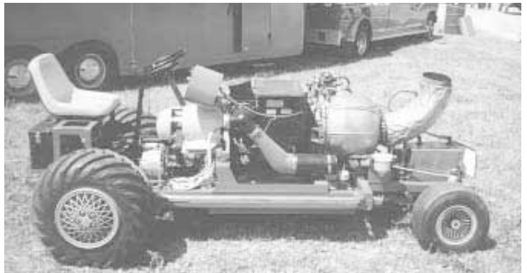
Wood coupled a golf cart front end and Deere lawn mower rear end with a powered it with a government surplus jet engine.
