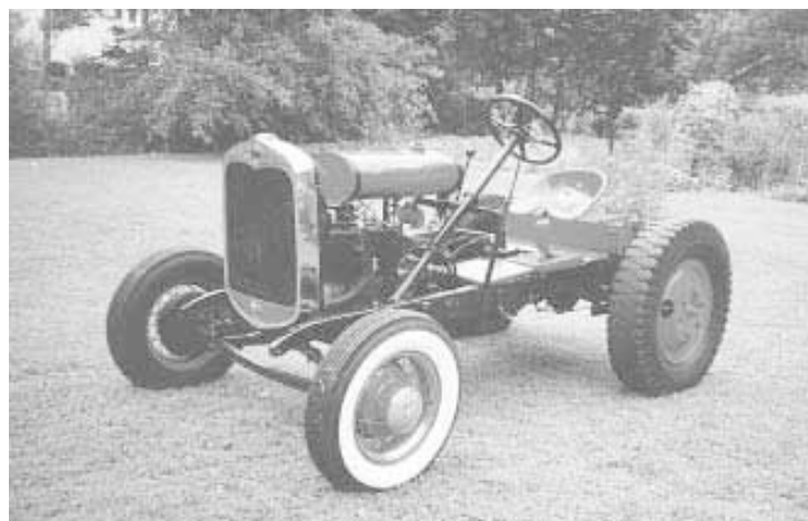
Model A car kept the original rear axle, 20-in. wheels, and frame. The whitewalls came off a Ford car, the radiator from a Model A, and the seat from a Ford 8N.
