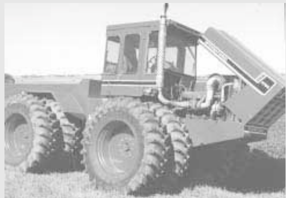
Photo above shows turbocharger intake and short section of flexible tubing used on exhaust system. Photo at right shows air cleaner on top of engine as well as the hydraulic oil filter.
