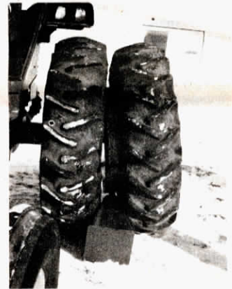
Drive forward over the wedge until you hear the wheel pop loose.
